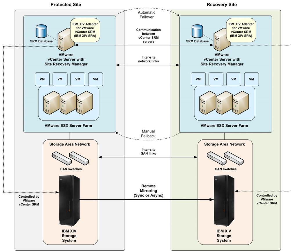
Figure 1. Protected and Recovery VMware site interaction with IBM XIV Storage
