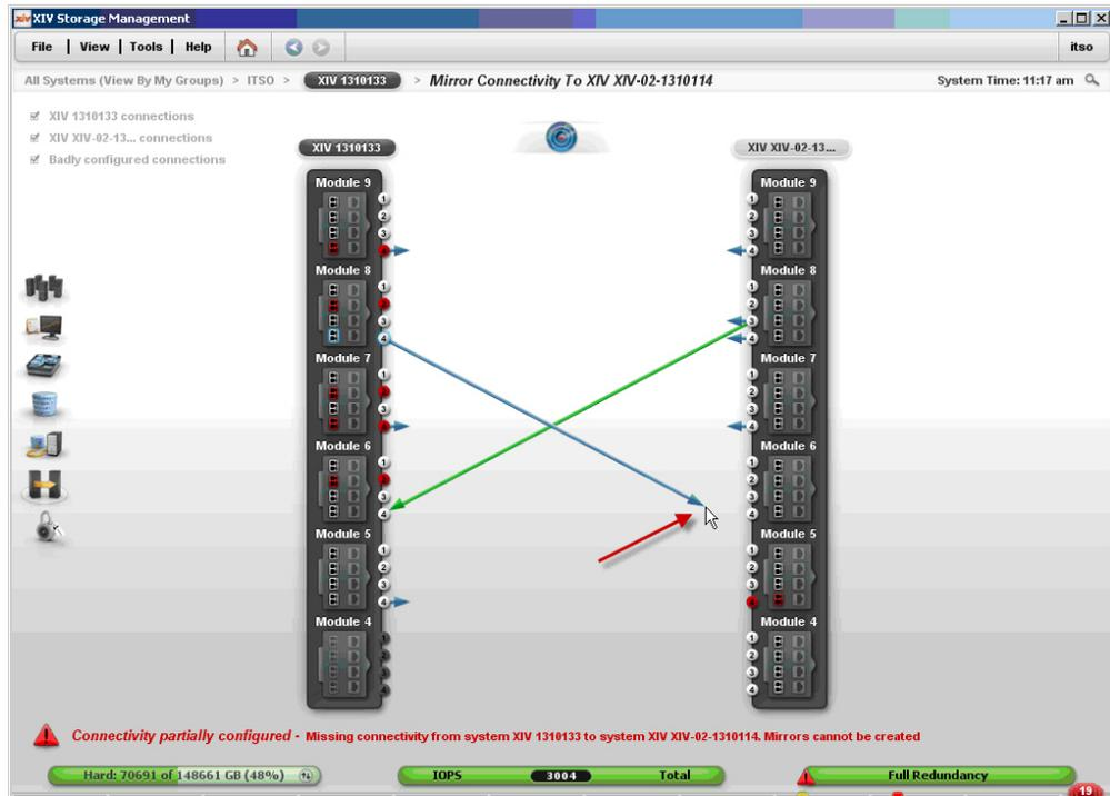
Figure 9. XIV Management GUI – Detected connections
